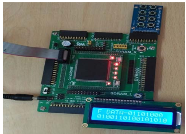
Fig. 5.5 Hardware Architecture of FM0/Manchester Encoder
