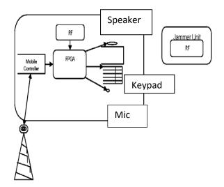
Fig 4.1 Schematic Diagram Of The Proposed Jammer
