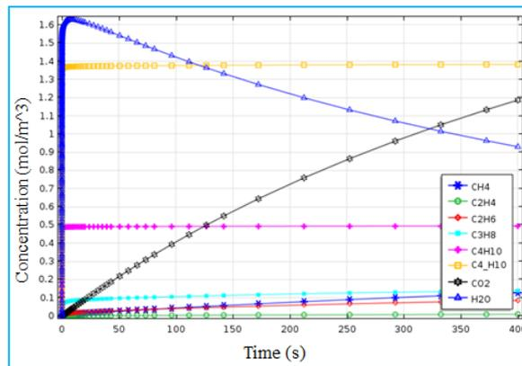
Figure 3: Production of methane, ethylene, ethane, n-butane, butane, carbon dioxide and water in the reactor.
