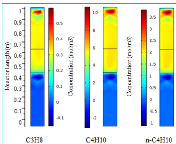
Figure 7: Concentration contour of species C<sub>3</sub>H<sub>8</sub>, C<sub>4</sub>H<sub>10</sub> and n-C<sub>4</sub>H<sub>10</sub>
