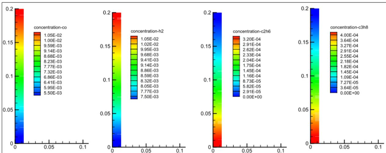
Figure 9: Concentration contour of CO, H<sub>2</sub>, C<sub>2</sub>H<sub>6</sub> and C<sub>3</sub>H<sub>8</sub> species within a reactor, from the work of Srinivas et al [14].
