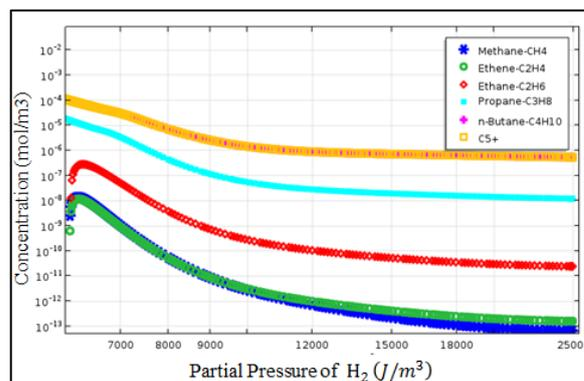
Figure 8: Effect of hydrogen partial pressure on the production of CH<sub>4</sub>, C<sub>2</sub>H<sub>4</sub>, C<sub>3</sub>H<sub>8</sub>, C<sub>4</sub>H<sub>10</sub> and C<sub>5+</sub> species.
