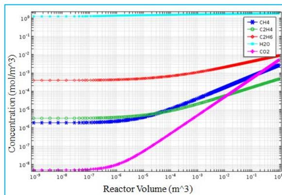
Figure 4: Concentration of species CH<sub>4</sub>, C<sub>2</sub>H<sub>4</sub>, C<sub>2</sub>H<sub>6</sub>, H<sub>2</sub>O and CO<sub>2</sub> against reactor volume.
