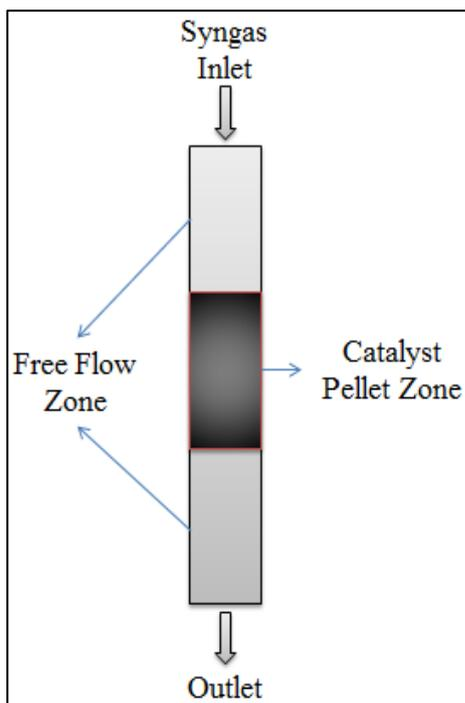
Figure 1: 2D Schematic of a fixed bed reactor tube
