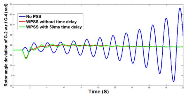
Fig-7 Rotor angle deviation of G-2 w.r.t G-4
