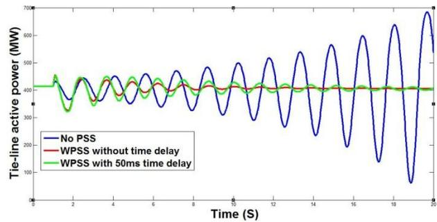
Fig-5 Tie-Line Active Power Flow
