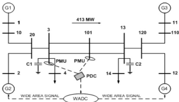
Fig-4 Kundur's Two Area Four Machine System
