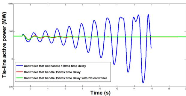
Fig-11 Tie-Line Active Power Flow with proposed controller, 150 ms delay
