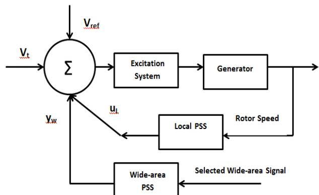
Fig-3 Configuration of the generator with PSS
