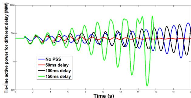
Fig-8 Tie-line active power flow for different delay
