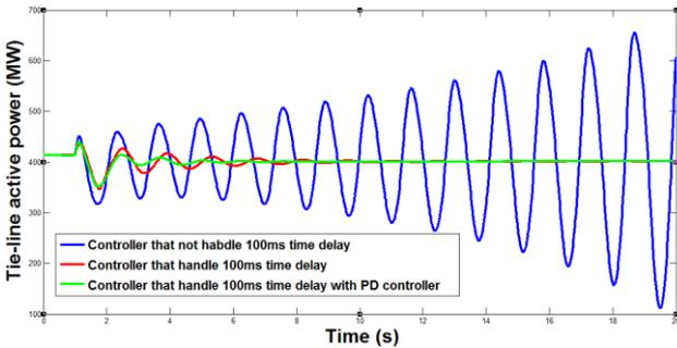
Fig-10 Tie-Line Active Power Flow with proposed controller, 100 ms delay
