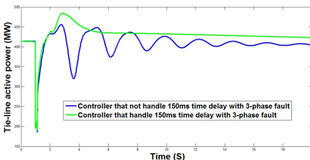
Fig-12 Tie-Line Active Power Flow with proposed controller, 150 ms delay
