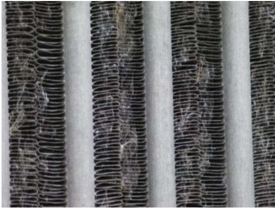
Fig.7. Particulate Fouling on Heat Transfer Fins
