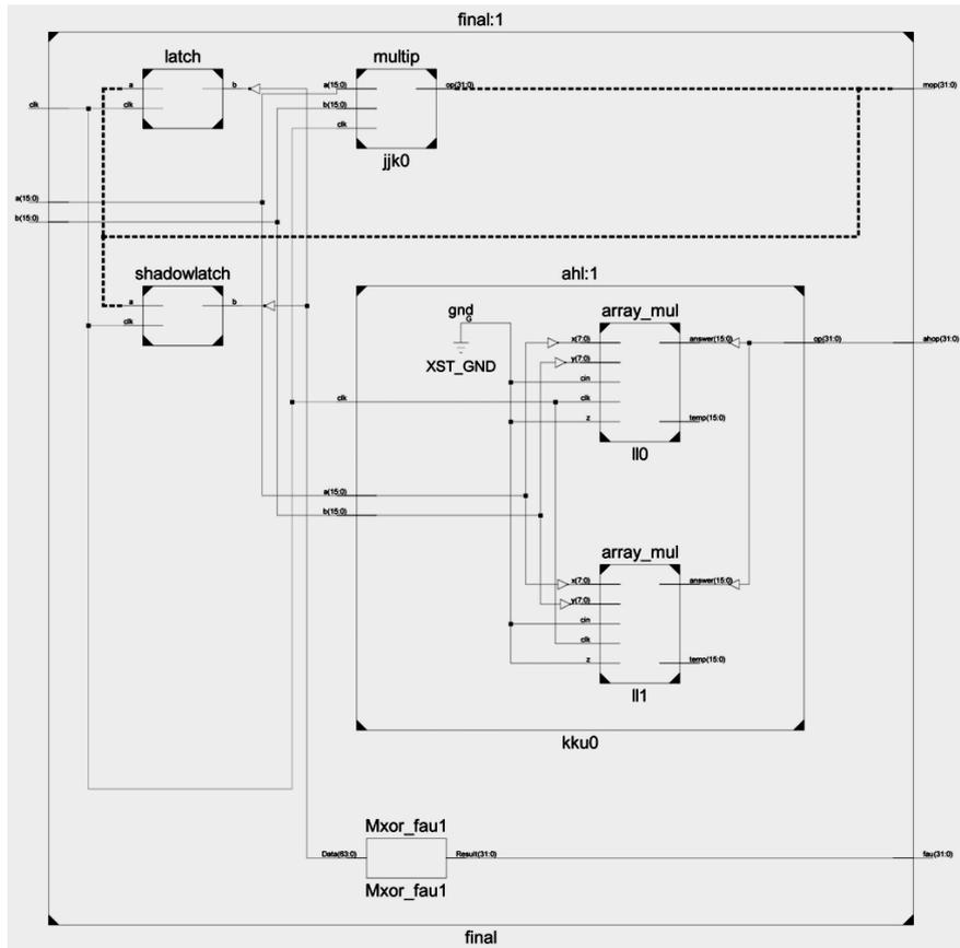
Figure: 4.1 RTL Schematic of Proposed Architecture .
