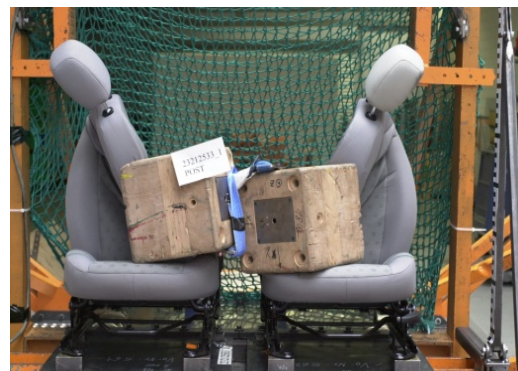
Test Procedure: Type-1(Rear seats without gap, without partitioning system)
