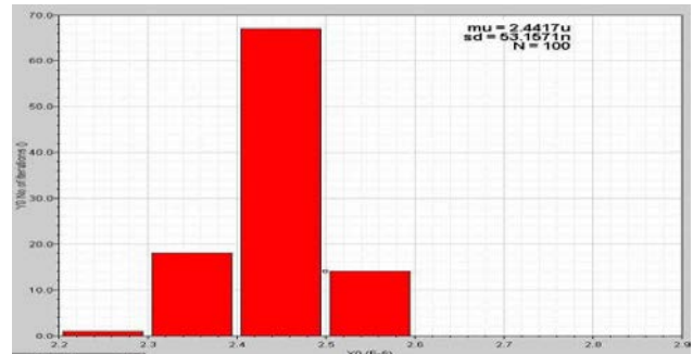
Fig. 3.1: Current source mismatch histogram
