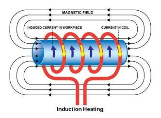
Fig 10: Working of induction hardening
