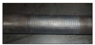
Fig 13: Induction hardened fork tube as specimen used for check of hardness after induction hardening.
