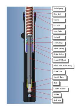
Fig 4: Damping mechanism of fork
