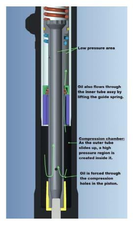
Fig 3a : Working of Inner Tube Compression
