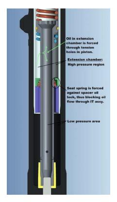
Fig 3b : Working of Inner Tube Compression
