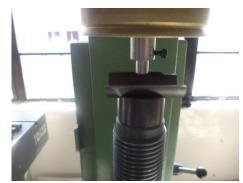
Fig 12: specimen mounted on hardness tester
