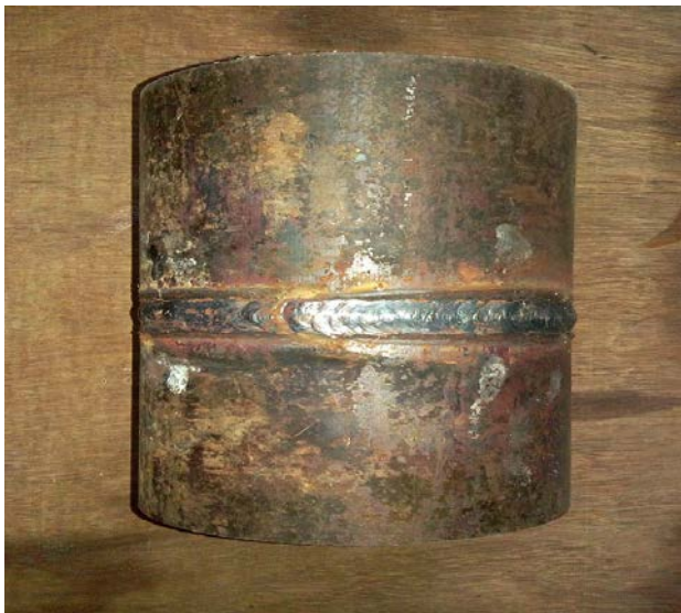
Fig. 6 work piece after welding
