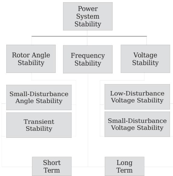
Fig. 1. Classification of Power System Stability
