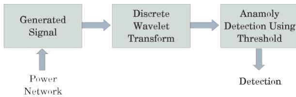
Fig. 2. Malicious Data Detection and Identification using Wavelet Analysis
