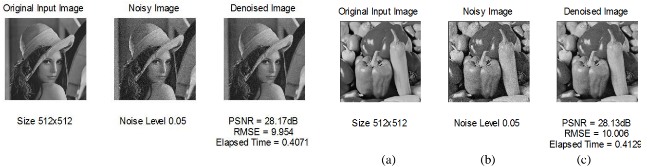
(a) (b) (c) Fig. 3.6 Lena and Peppers Images of 512x512 Size (a) Original Input Image, (b) Noisy Image, (c) Denoised Image with Noise Level 0.05
