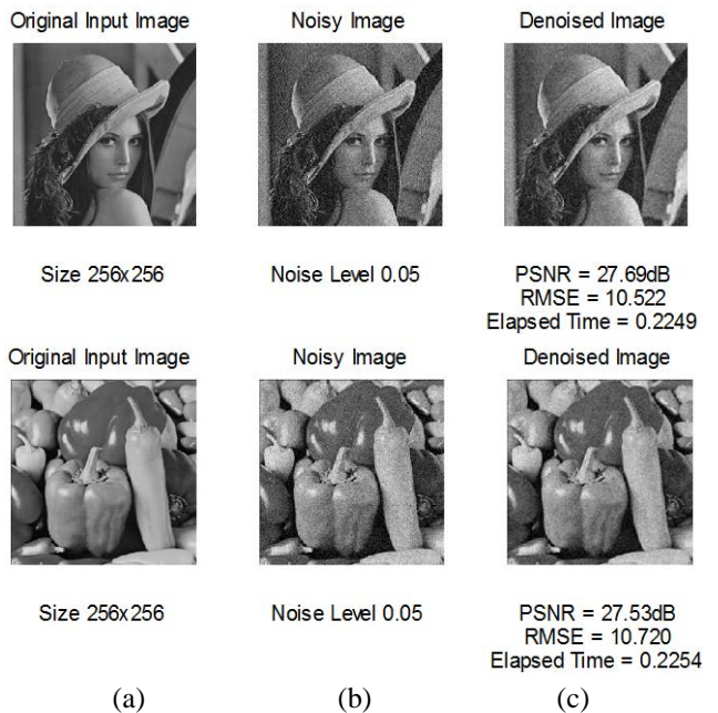
Fig. 3.5 Lena and Peppers Images of 256x256 Size (a) Original Input Image, (b) Noisy Image, (c) Denoised Image with Noise Level 0.05
