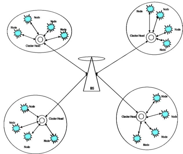
Fig. 2.1. Clustered Architecture Illustrating data aggregation.
