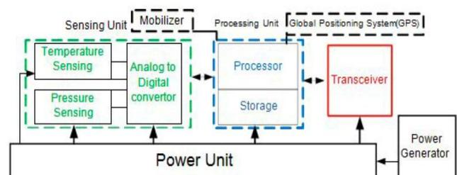
Figure 1.2: Sensor Node's Architecture
