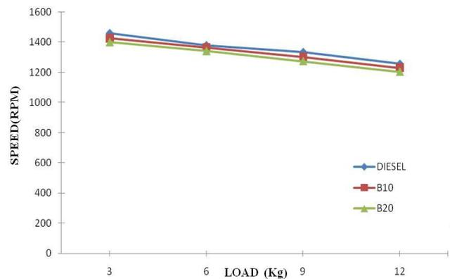
Fig.8 Variation of Speed for blended with diesel
