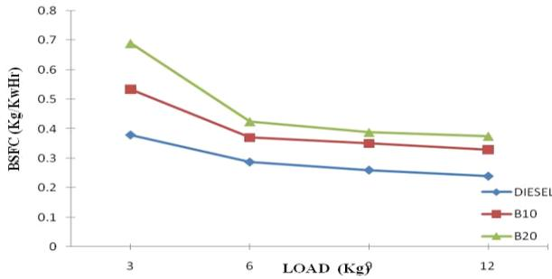
Fig.2 Variation of BSFC for blended with diesel
