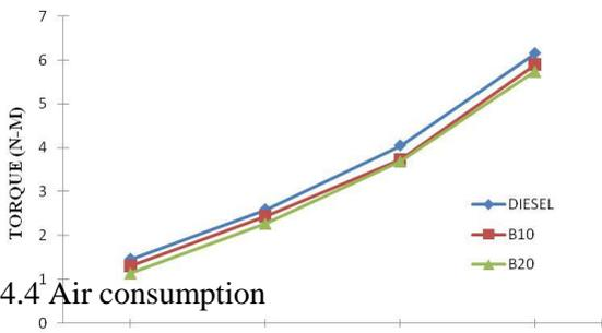
Fig.3 Variation of Torque for blended with diesel
