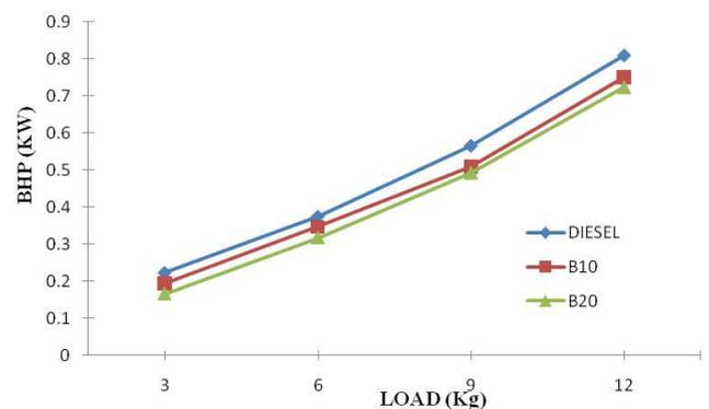
Fig.1 Variation of BHP for blended with diesel
