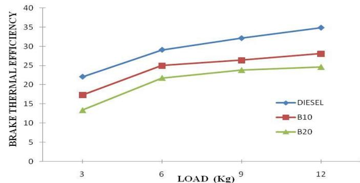
Fig.5 Variation of Brake thermal efficiency for blended with diesel
