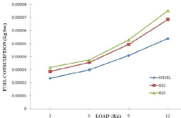
Fig.6 Variation of Fuel consumption for blended with diesel
