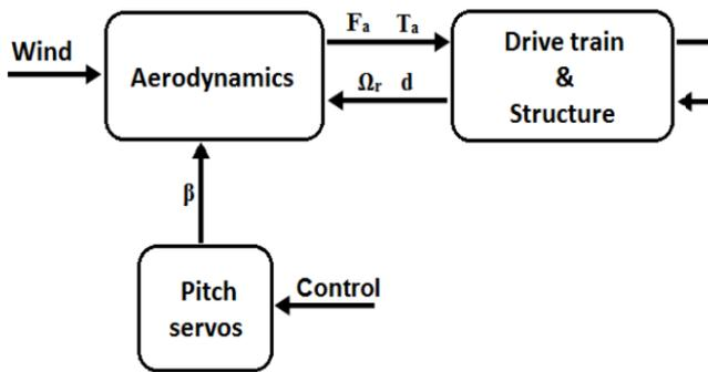
Figure 1.2 Sub System-level block diagram of a variable speed variable – pitch (VS-VP) Wind Turbine.
