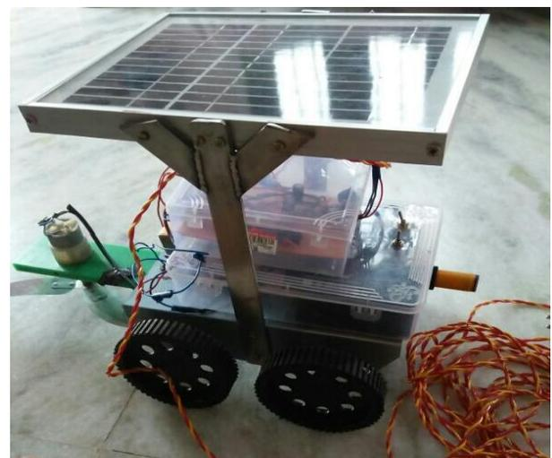
Fig 4.1 Hardware implementation of Fully automated solar grass cutter.
