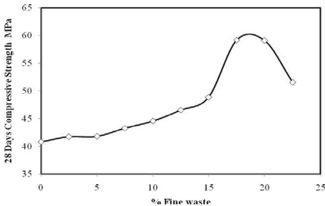
Fig. 2 Effect of substituting fine alum waste for sand on the 28 days strength
