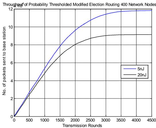
Fig. 4.5 Base Station Throughput vs Rounds
