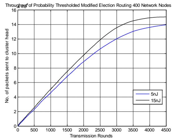
Fig. 4.4 Cluster Head Throughput vs Rounds
