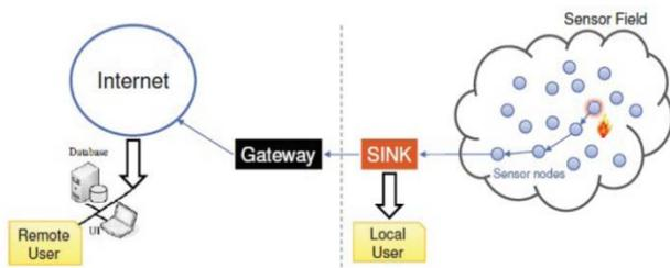
Figure 1.1 Basic WSN network structure.
