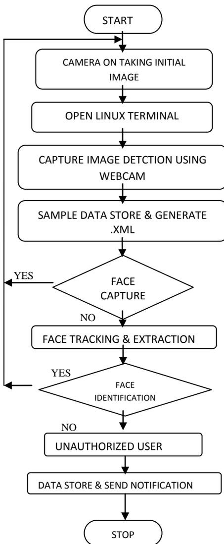
Fig. 3. General System Flowchart
