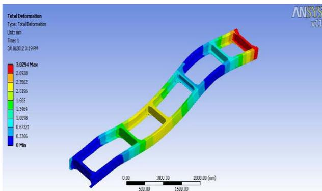
Fig.8 Displacement in chassis frame
