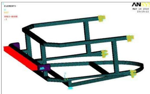
Fig.6 Car frame with imposed boundary conditions
