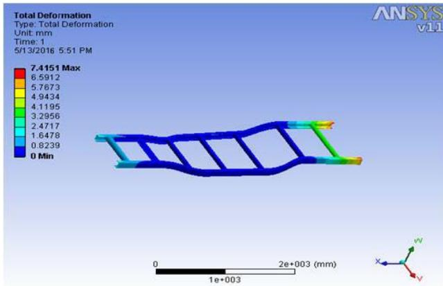
Fig.5 Load applied on chassis
