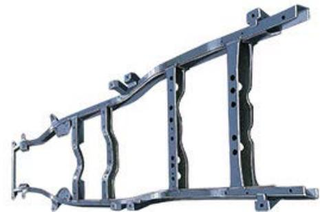
Fig 1:Ladder frame chassis
