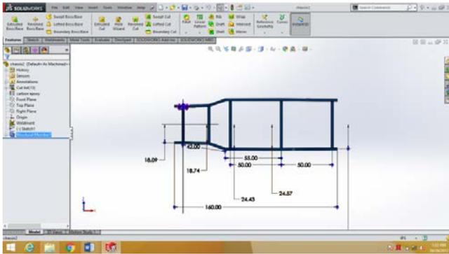
Fig.3 chassis design with dimensions
