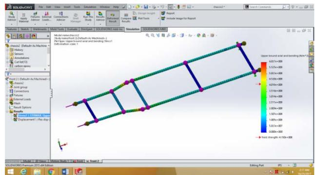
Fig.8 stress plot for chassis during front collision
