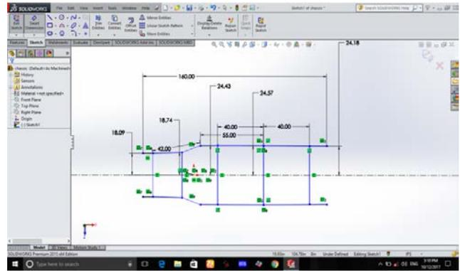
Fig 12 New chassis design
