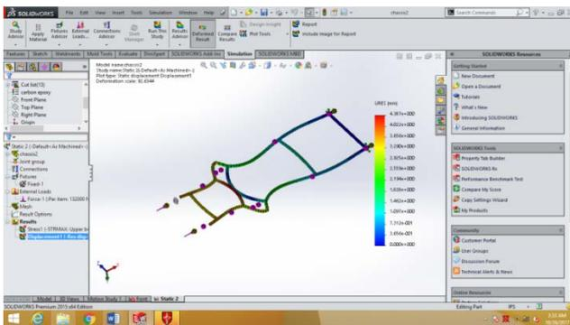
Fig. 11 Deformed Chassis with 99.152 scale
