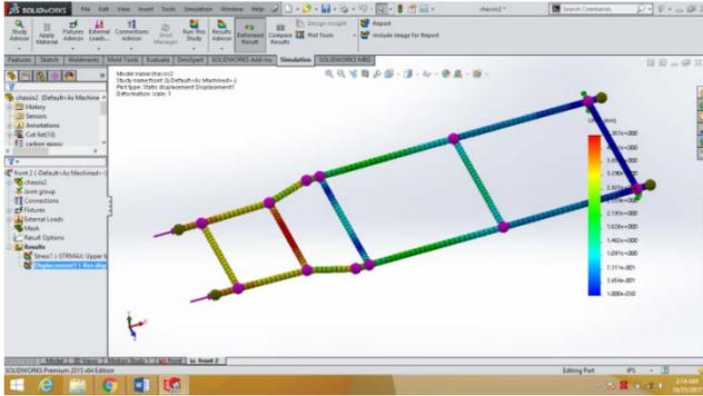
Fig.10 displacement during front collision
