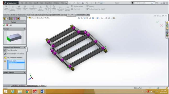
Fig.7 applying fixtures
