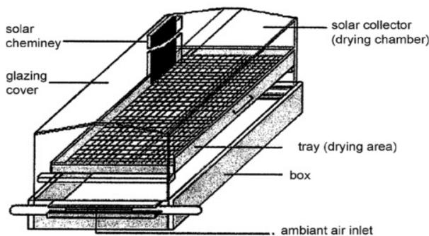
Fig. 3.1 : Natural convection direct solar drier [11]
