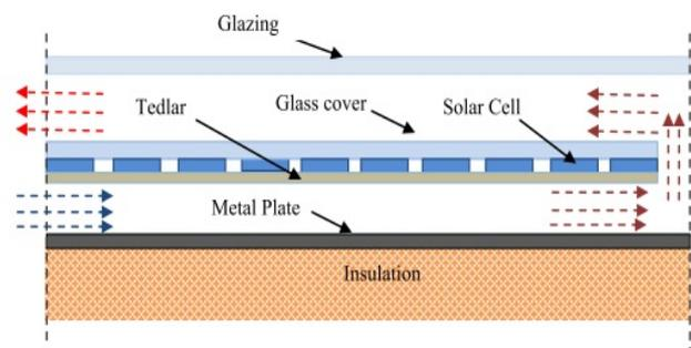
Fig. 3.2 : Hybrid PV/T solar collector [14]
