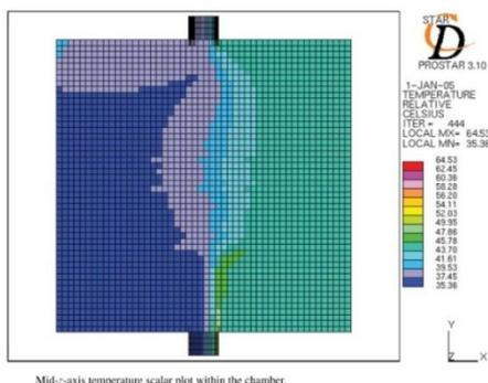
Fig. 5.1 : Unsymmetric temperature profile of air flow in drying chamber [16]
