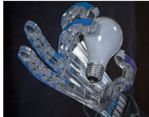
Fig 4.2:-Robotic hand operated by compressed air
