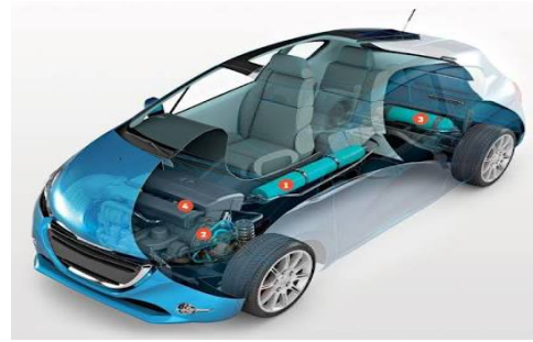
Fig 4.1:- Compressed Air Vehicle
