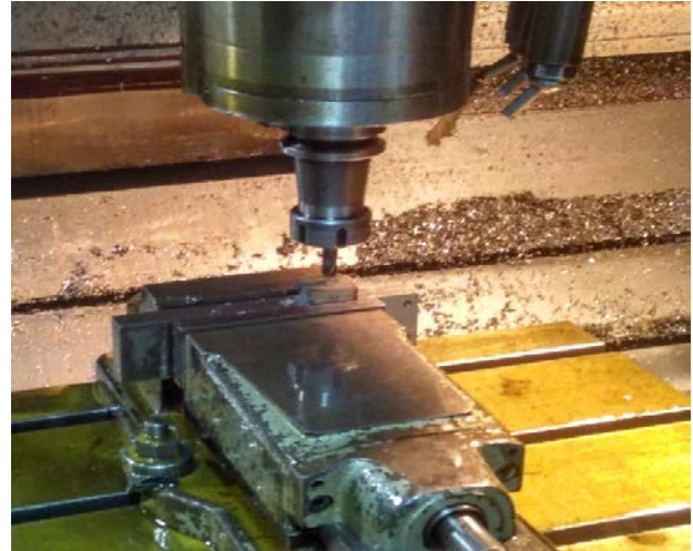
Fig.4.1 End Milling on VMC
