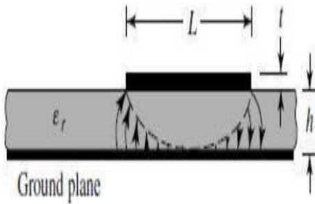
Figure: 1.2 Side view of Microstrip Patch Antenna
