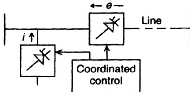
Fig. 3.4: Combined Series-Shunt Compensator
