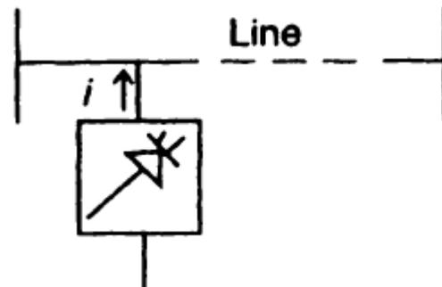
Fig. 3.1: Shunt Compensator
