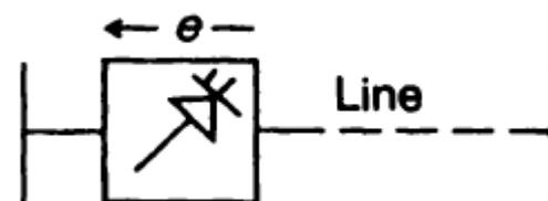
Fig. 3.2: Series Compensator
