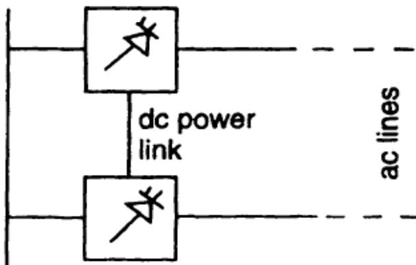
Fig. 3.3: Combined Series-Series Compensator
