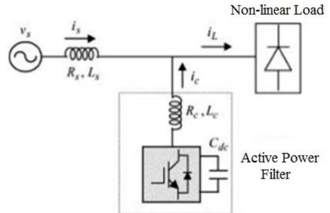
Fig. 4.1: General Block Diagram of Shunt Active Power Filter
