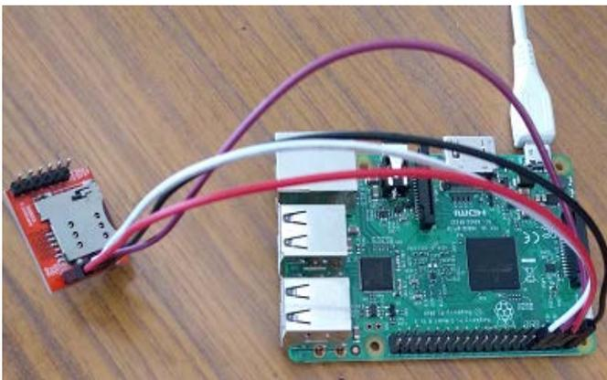
Fig. 5.3 Interfacing GSM to Raspberry pi
