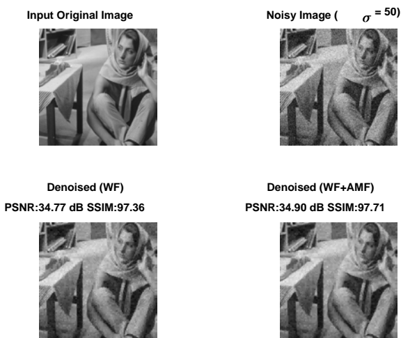
Figure 4.3 Result with Wavelet and Wavelet + AMF of PSNR and SSIM for Barbara image on \sigma = 50
