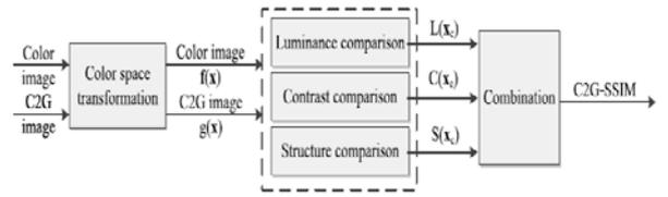
Fig. 1. Three-stage structure of C2G-SSIM.
