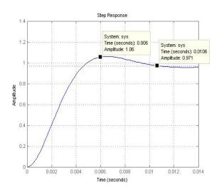
Fig.3 Response of motor with P controller
