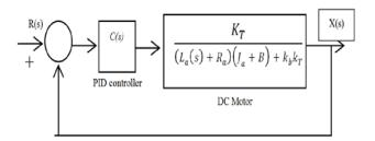
Fig.1 PID DC motor speed control system block diagram.
