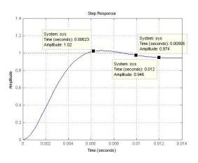
Fig.5 Response of Motor with PI Controller
