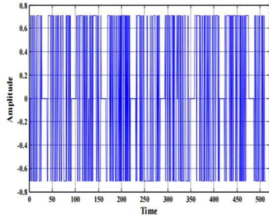
Figure 2: Transmitted QPSK symbol of MIMO-OFDM ( $N_{Tx} \times N_{Rx}$ ) system.
