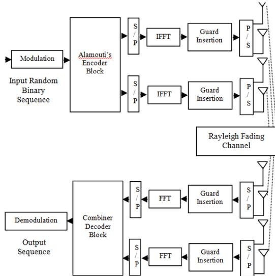
Figure 1: System Model of MIMO-OFDM system
