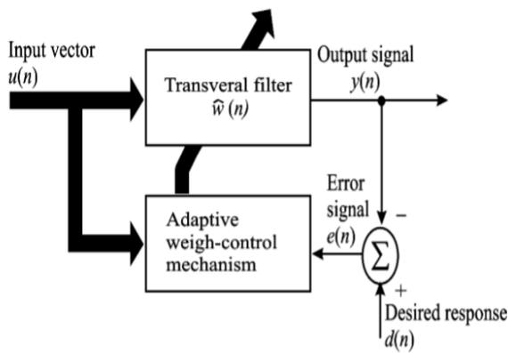
Figure 3: Block diagram of adaptive transversal filter
