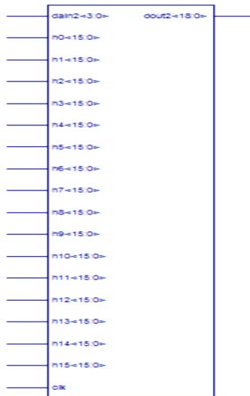
Figure 5: View Technology Schematic of 16-tap FIR Filter using DA Technique
