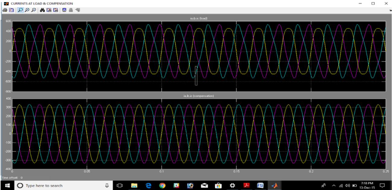
Figure 4.1 Three-phase source current waveforms obtained by A, B, C phases.
