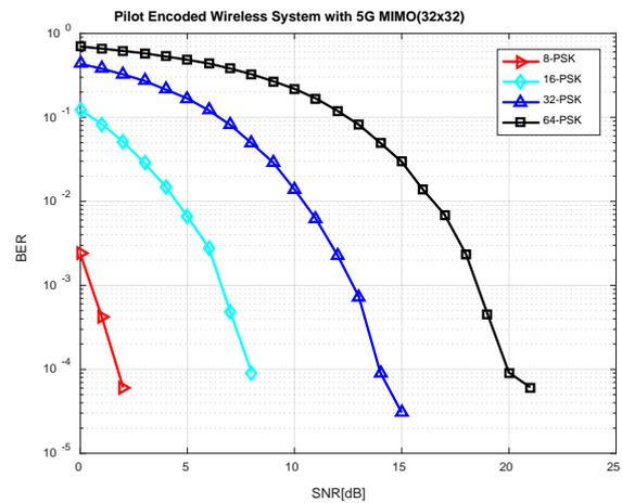
Fig. 4.5 BER Vs SNR Curve for 5G MIMO with Antenna Configuration Tx=32 and Rx=32.
