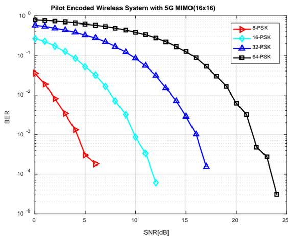
Fig. 4.4 BER Vs SNR Curve for 5G MIMO with Antenna Configuration Tx=16 and Rx=16.
