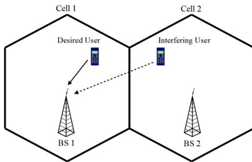
Figure 2.1 Pilot contamination examples when both users transmit mutually non-orthogonal training sequences.
