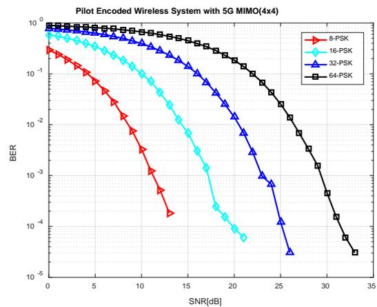
Fig.4.1 BER Vs SNR Curve for 5G MIMO with Antenna Configuration  $T_x=4$  and  $R_x=4$ .
