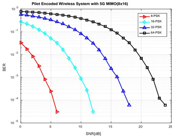
Figure 4.3 BER Vs SNR Curve for 5G MIMO with Antenna Configuration Tx=8 and Rx=16.
