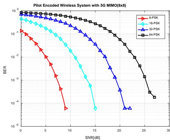
Fig. 4.2 BER Vs SNR Curve for 5G MIMO with Antenna Configuration  $T_x=8$  and  $R_x=8$ .
