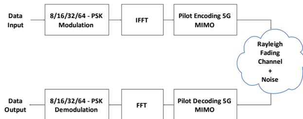
Figure 3.1 Block Diagram.
