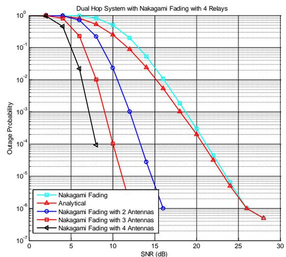
Fig. 4.3 Outage Probability of Dual Hop Cooperative Relay system with multiple antennas and  $R=4$
