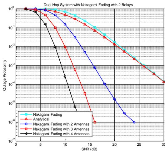
Fig. 4.2 Outage Probability of Dual Hop Cooperative Relay system with multiple antennas and  $R=2$
