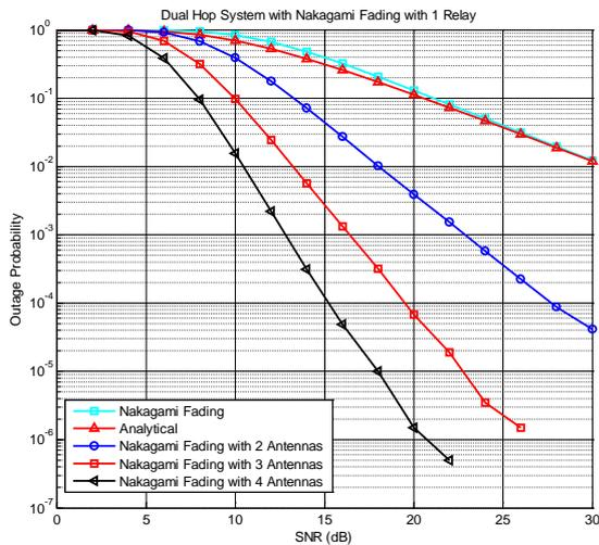
Fig. 4.1 Outage Probability of Dual Hop Cooperative Relay system with multiple antennas and  $R=1$
