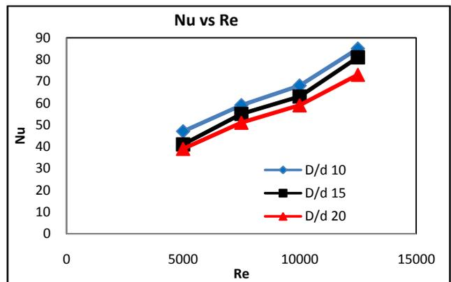
4.2 Variation of Nu with Re for different D/d ratio for turbulent flow
