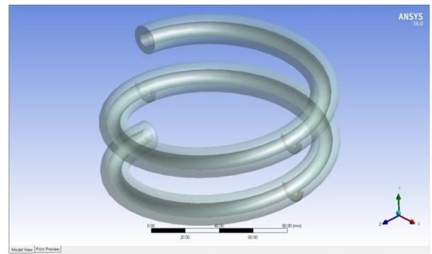
Figure 3.4: Geometry showing hot fluid region, cold fluid region, Baffles
