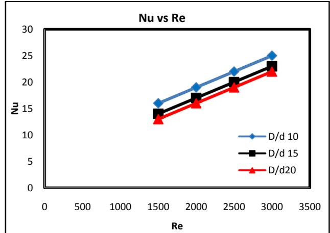
4.1 Variation of Nu with Re for different D/d ratio for laminar flow
