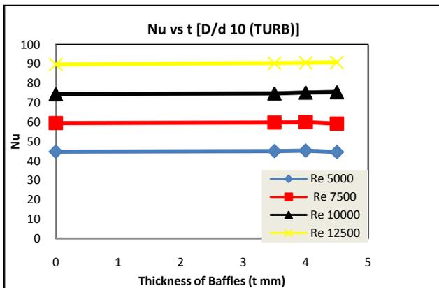
4.4 Variation of Nu with thickness of baffle  $t$  (mm) for  $D/d=10$  turbulent flow for various Re values.
