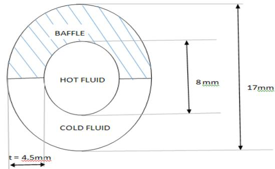
coil tube in tube heat exchanger at the baffle
