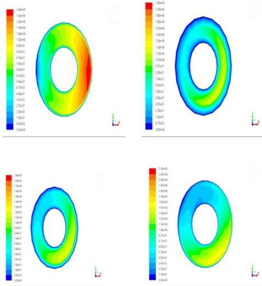
4.3 Velocity contour for cold fluid outlet in the increasing order of thickness of baffle
