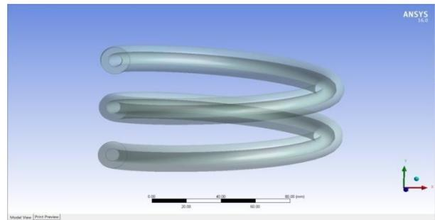
Figure 3.3: Geometry showing cold fluid region
