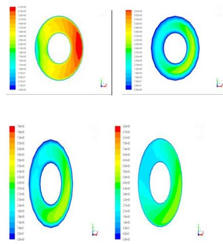
4.6 Velocity contour for cold fluid outlet in the increasing order of thickness of baffle
