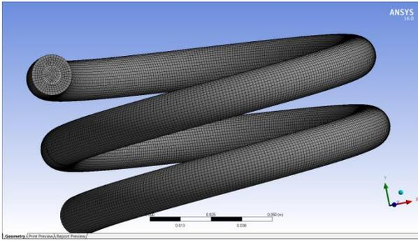
Figure 3.5: Image of geometry which is meshed fully
