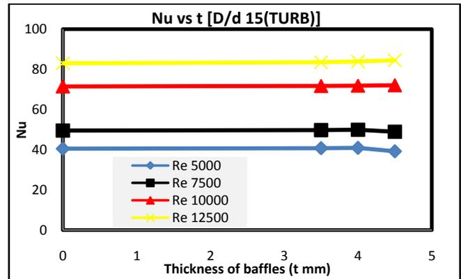
4.5 Variation of Nu with thickness of baffle  $t$  (mm) for  $D/d=15$  turbulent flow for various Re values
