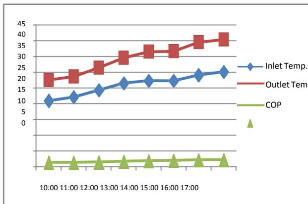
The ambient temperature started at 21°C (10 AM), increasing the highest value 30.30°C at 5 pm. Basic soil temperature at 3m depth was constant at 24.2°C. Temperature of the air at the outlet varying from 27.53°C to 40.36°C. ETHE was able to raise the ambient air
