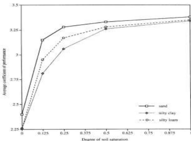
Fig.2.2: Variation of the average COP vs soil degree of saturation.
