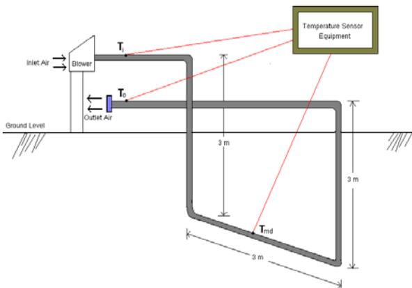
Fig. 4.1: Schematic Representation of Experimental Set up
