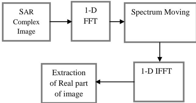
Fig 2: block diagram of FFT
