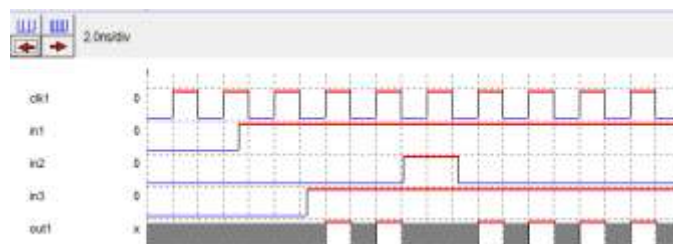
Figure 8: Input output waveform for MTCMOS.
