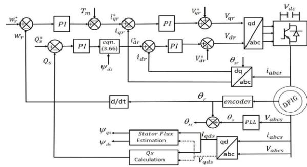
Figure 7: Block diagram of RSC control system
