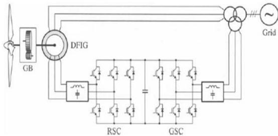
Figure 3: Variable speed with reduced capacity configuration
