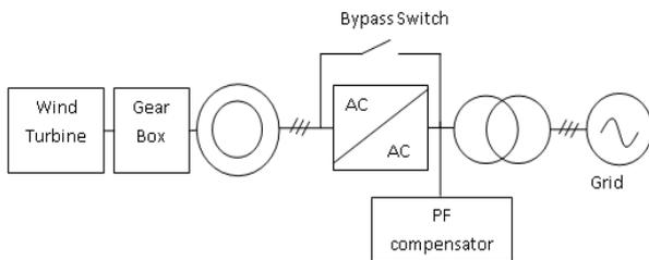
Figure 4: Variable speed with full capacity configuration
