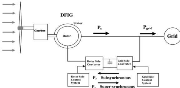
Figure 1: DFIG based Wind Turbine Generator System
