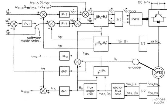
Figure 5. Stator flux oriented control scheme
