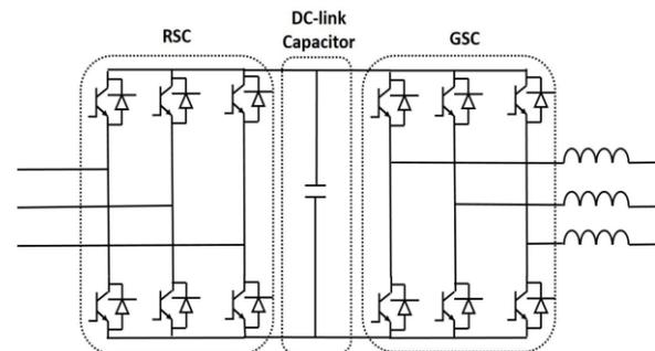
Figure 2: Power converter of the DFIG
