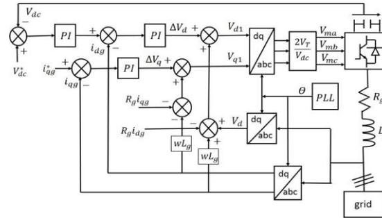
Figure 6: Grid side VSC control scheme
