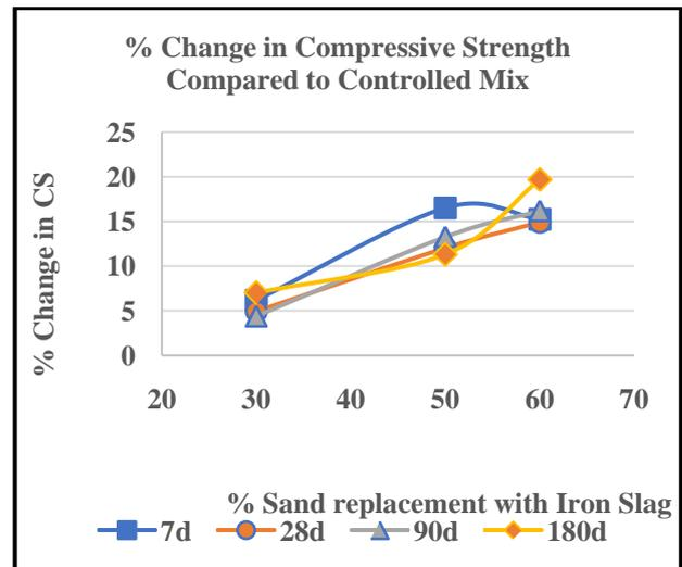
Figure- 5: Percent Change in Compressive Strength compared to Controlled Mix
