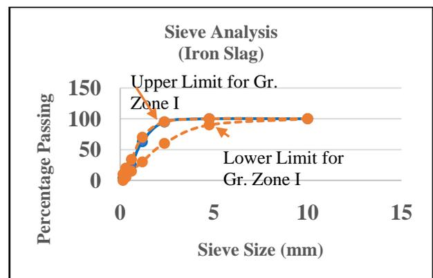
Figure -3: Sieve Analysis of Iron Slag
