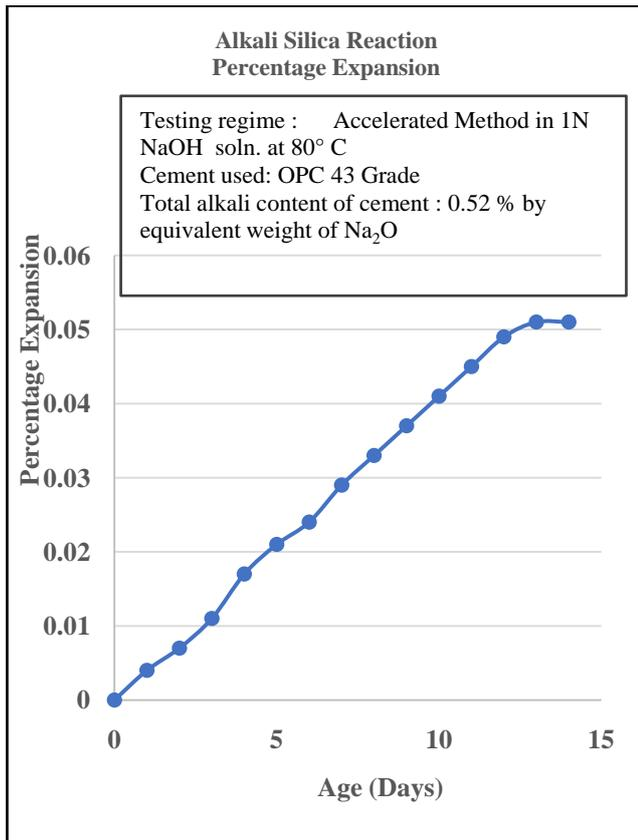
Figure-1: Alkali Silica Reactivity Test on Coarse Aggregates
