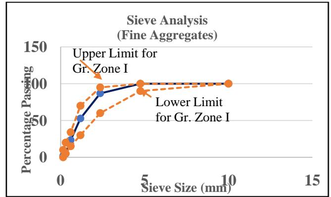
Figure -2: Sieve Analysis of Fine Aggregates
