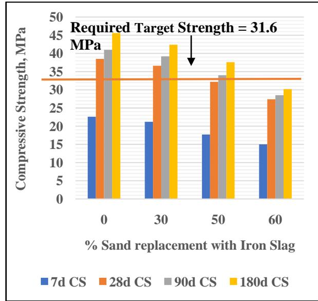
Figure- 4: Compressive Strength of Concrete with varying % of Iron Slag
