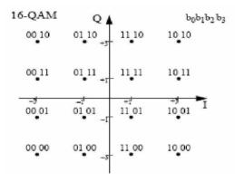
Fig. 3.2 Constellation Diagrams for 16 QAM.
