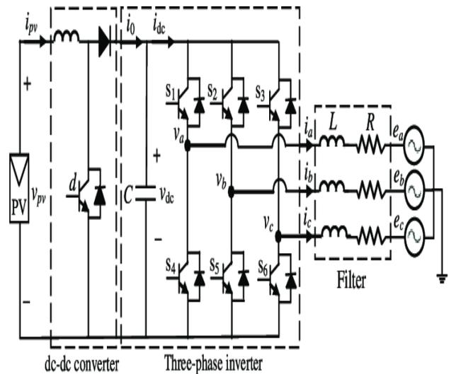
Fig 2.1 Grid Connected PV System Structure.
