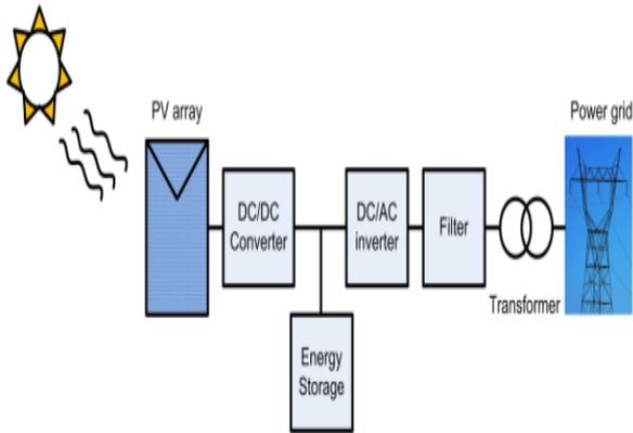
Fig. 1.1 Components of a Grid Connected PV System.
