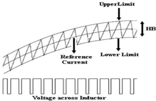
Fig 2.2 Hysteresis Current Control Operation Waveform
