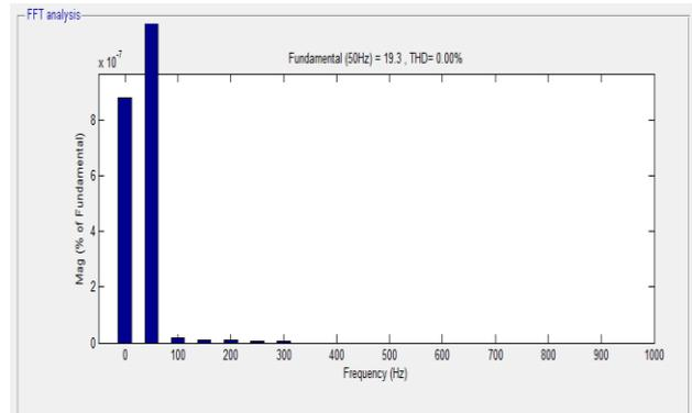
Fig. 4.7 Total Harmonic Distortion reduced from 30 % to 0%
