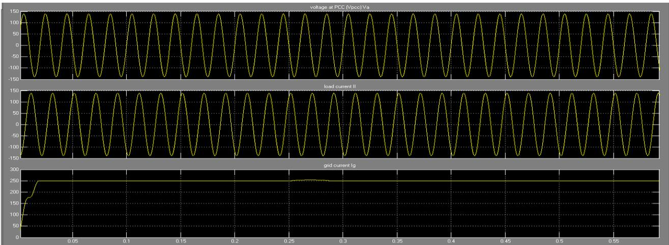
Fig.4.5 Source Voltage, Source Current and Grid DC Voltage in Grid Mode.
