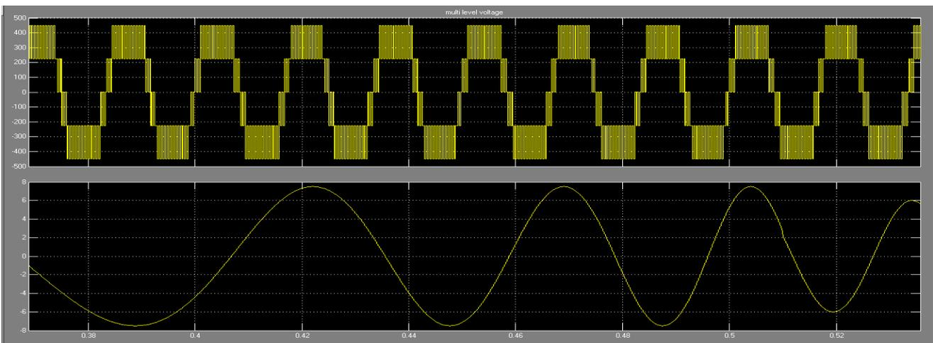
Fig.4.8 Multi Level Voltage and Stator Current in Grid Connected Mode.
