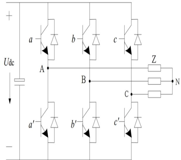
Fig. Three- phase voltage source circuit.
