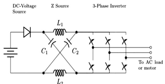
Fig. 1.2 Z-Source Inverter.
