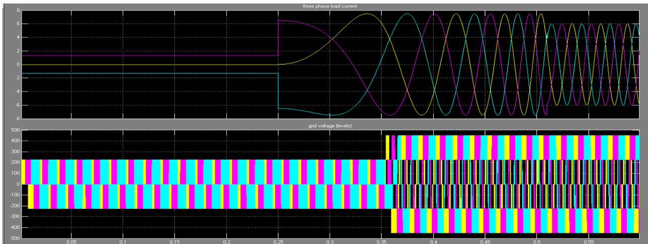
Fig.4.6 Three Phase Load Currents and voltages in Grid Connected Mode.
