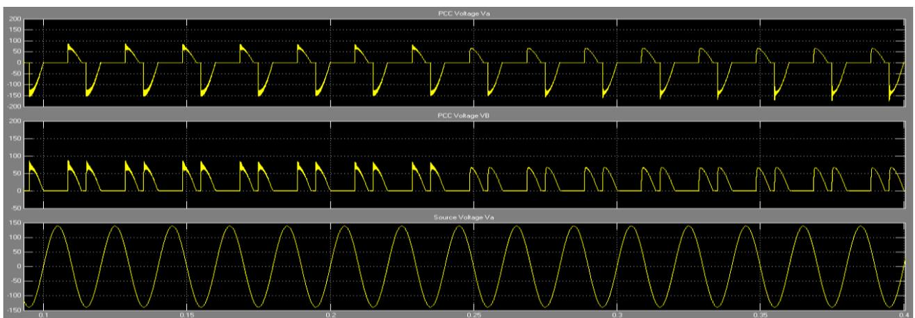
Fig.4.3 PCC and Source Voltages in Islanded Mode.
