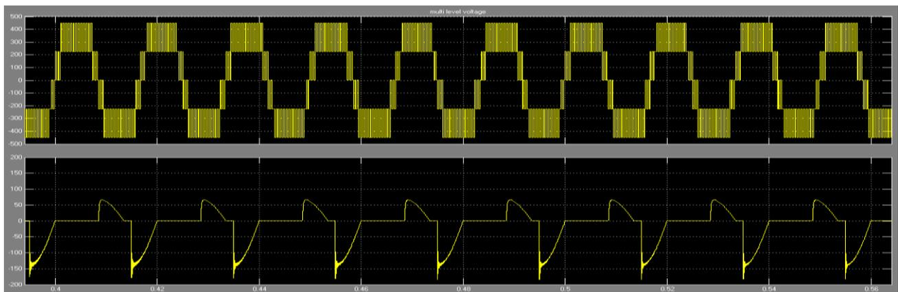
Fig.4.9 Multi Level Voltage and Stator Current in Islanded Mode.
