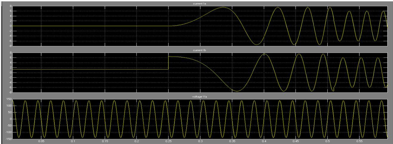
Fig.4.1 Grid Connected Mode Stator Current and Source Voltage.
