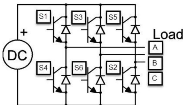
Fig. 1.1 Traditional Voltage-Source Inverter
