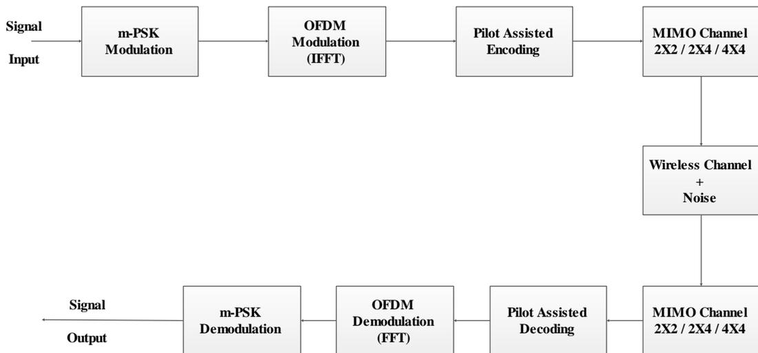
Fig.3.1 Block diagram of proposed work.
