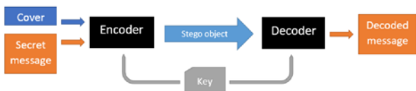
Fig.2.2 A simple model of Steganography
