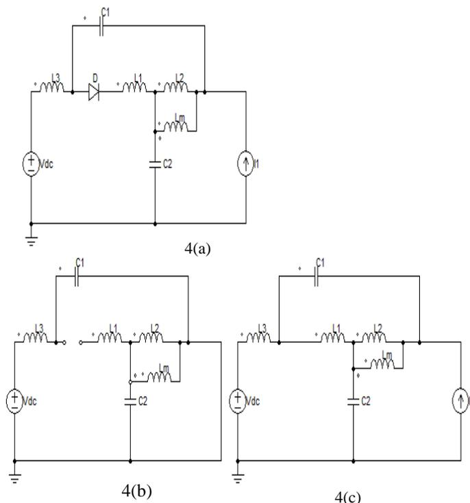
Fig.4(a).Equivalent circuit, 4(b). Shoot through state, 4(c).non-shoot through state
