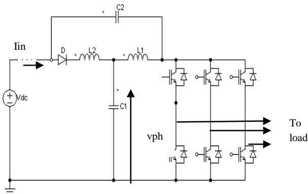
Fig 3. Improved Trans-Z-source inverter
