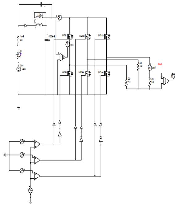
Fig.5.Simulation of improved trans-Z-source inverter
