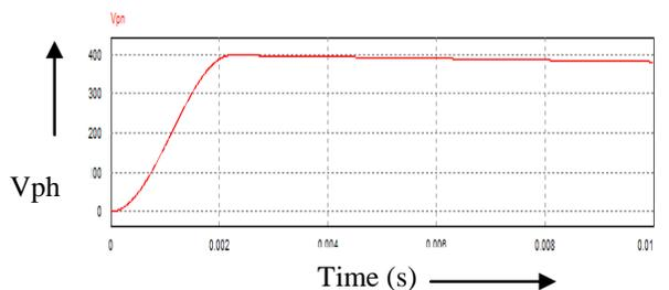
Fig. 5(b). Simulation graph of inverter voltage
