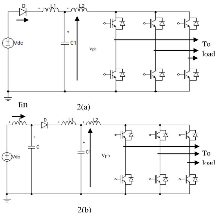
Fig.2.(a) Trans-Z-source inverter or T-source inverter.Fig.2.(b) Trans-Z-source inverter with LC filter
