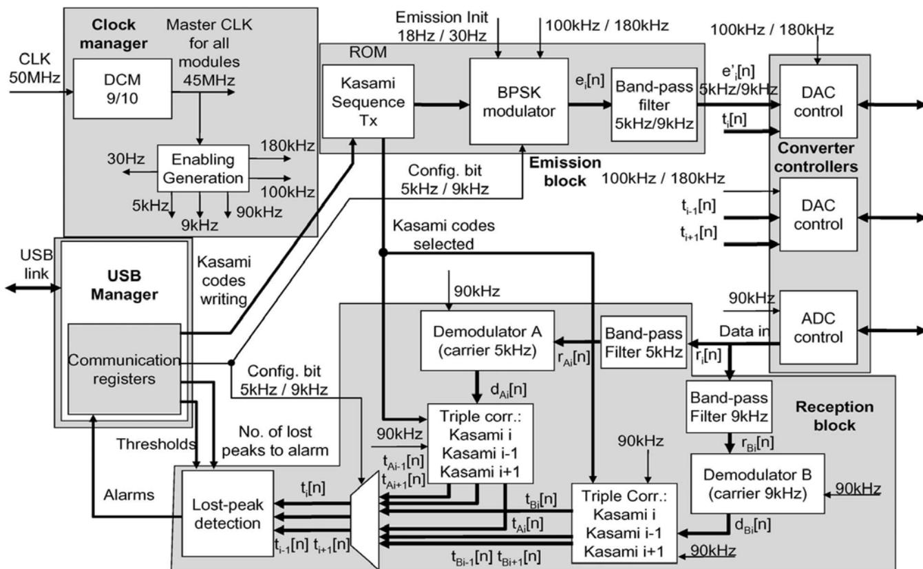
Fig.4. Global block diagram of the hardware implementation inside the FPGA device.
