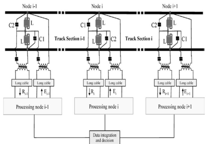
Fig. 1. Global structure of the proposed track circuit.
