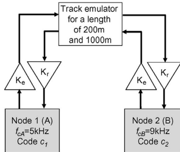
Fig.3. Experimental setup used for validation
