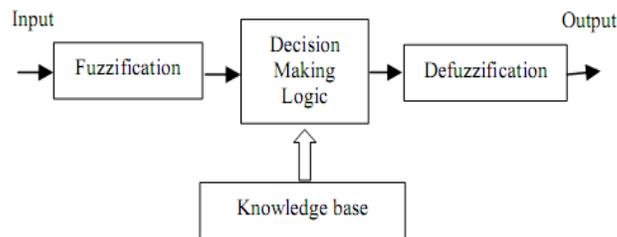
Fig. 5. Block Diagram of Fuzzy logic system
