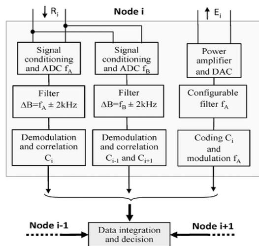
Fig.2.Detailed block diagram of a processing module for a generic node *i*
