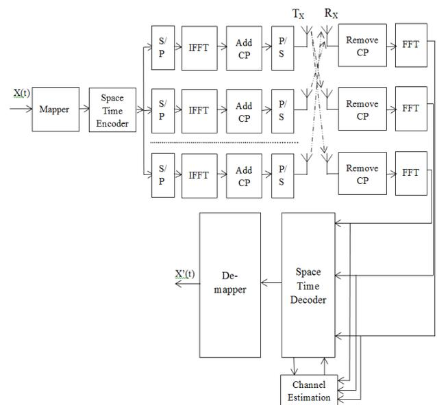
Figure 2: MIMO-OFDM System Models with Channel Estimation Technique
