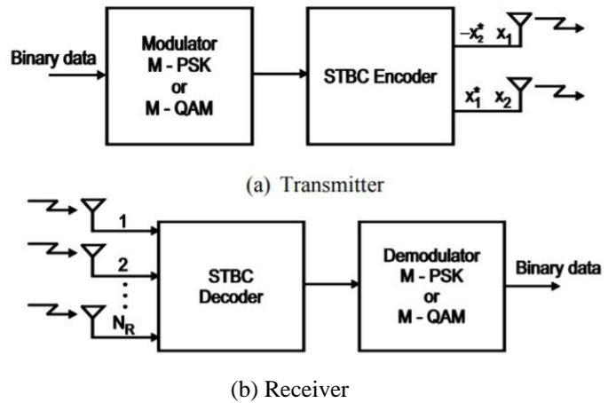
Figure 1: A MIMO communication system with STBC Code
