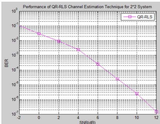
Figure 4: Performance BER for 2x2 MIMO-OFDM Systems
