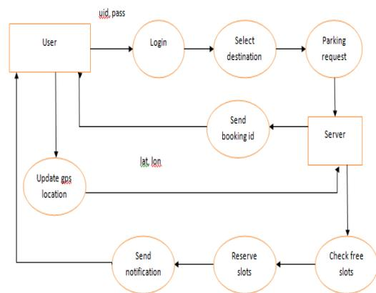
Figure 4: Level 2 Dataflow Diagram.
